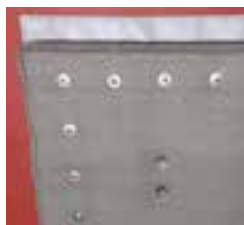
Gas turbine insulator panel
